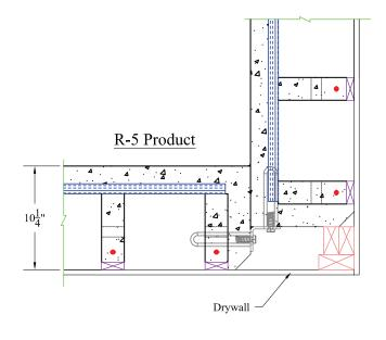
Cut Pressure Treated Lumber (2x4) As Shown
