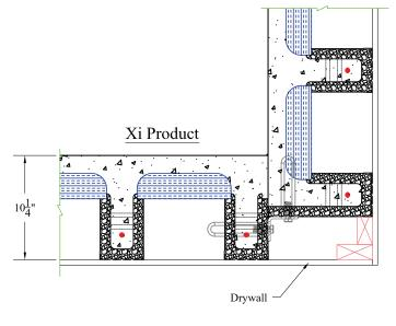
Cut Pressure Treated Lumber (2x4) As Shown
