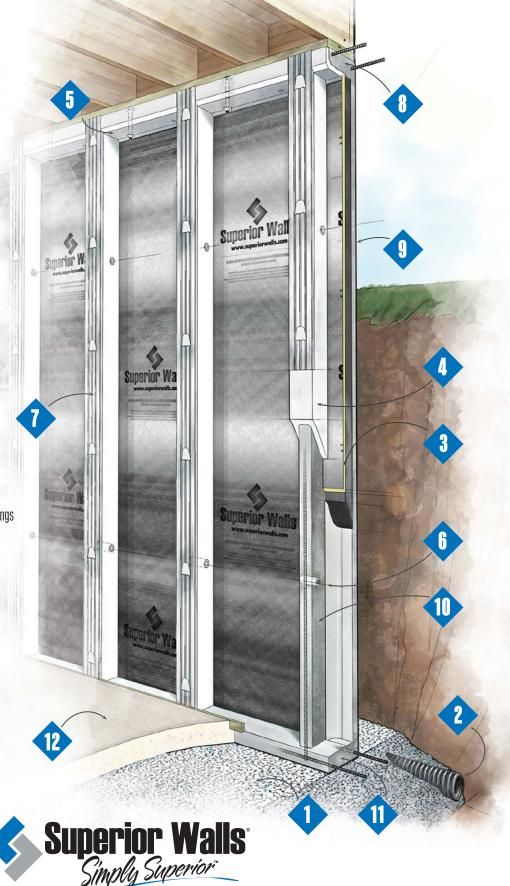
Special Note: Items #1,2 &12 as well as the joist/flooring system are provided on site, per Superior Walls specifications, by builder and contractors as an integral part of the Superior Walls foundation system.
